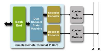
Designed from ground up for use in space, Sital's BRM1553ERL IP core, offers uniquely compact, robust and reliable BC, RT, MT solutions for any FPGA and ASIC device. The core implements special means for overcoming problems related to radiation and harsh conditions often found in space applications.
