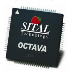
The OCTAVA™ family of Mil-Std-1553 devices integrate Mil-Std-1553B protocol engine, a dual 5-volt transceiver, memory management, processor interface logic, and 4K or 64K words of RAM in a 72 Pin Plastic Quad Flat Pack (PQFP) package.
