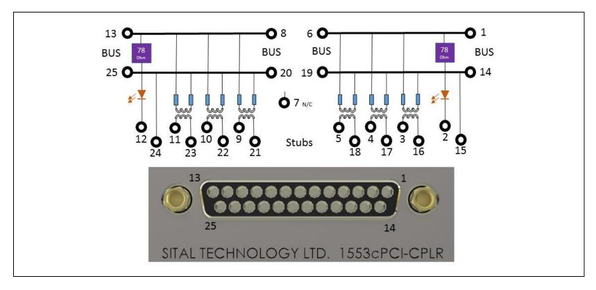
The dual 3-stub coupler (as seen in the above diagram) connects with the pins of the 25-Pin D-Type female connector.
