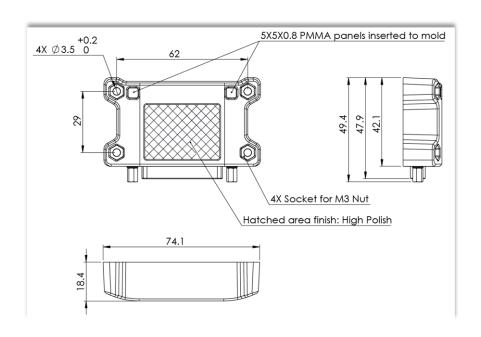
Material: Black, TPU90 Shore A, Over molded on Electronics.
