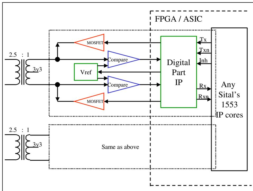
The transformer configuration is to have a center tap powered by the 3.3v power supply. The transformer's turn ratio should be a standard MIL-STD-1553 1:2.5 transformer. Each MOSFET driver pulls current in one half of the transformer, yielding an amplifying turn ratio of x5. The actual transformer voltage drop on each half is about 2v. When amplified by 5, the output transformer voltage of both halves is thus about 20v peak to peak.
