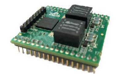
The BRD1553XVR unit is intended for Mil-Std-1553 IP cores evaluation and development of 1553 applications. The BRD1553XVR unit can be used for PCB applications containing FPGAs that need the MIL-STD-1553B but do not have a transceiver on board. The unit also includes 2 transformers, eliminating any need for any additional 1553 components. Using BRD1553XVR makes the IP Core evaluation and 1553 applications simple and easy.
